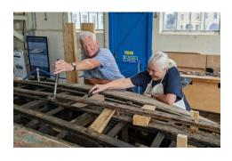
cut the through bolts along the keel and hog so that they can split them in order the make new for the rebuild. The current keel and hog are quite
